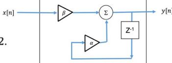
(iii) Find the transfer function G[z] of the system for  $\alpha = 0.8$ ,  $\beta = 0.2$ .
