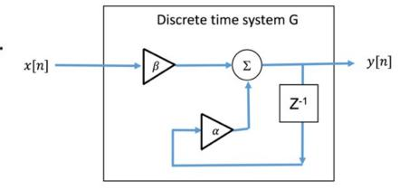
(ii) Derive the output sequence  $y[0], y[1], \dots, y[9]$  given that  $\alpha = 0.8, \beta = 0.2,$  x[0] = 0 and x[n] = 10 for  $n \ge 1$ .
